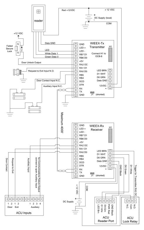
Figure 106 - CWIEEX - Coaxial Transmitter/Receiver Connections
