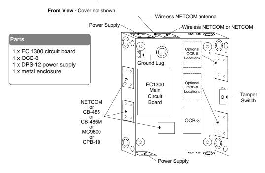
Figure 10 - EC 2000 with Circuit Board Mounting Positions
