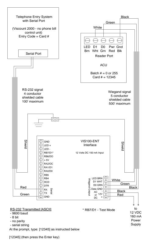
Figure 119 - VIS100 SES Connections
