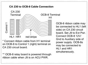
Figure 112 - Pre-alert Relay CA 4300/OCB-8 Connections
