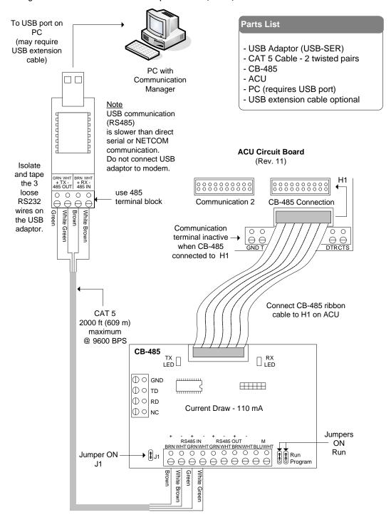
Figure 50 - Single ACU Communication - USB Adaptor/CPB-10 (RS232)
