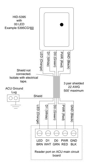
Figure 87 - HID 5365 / 6005 Wiring
