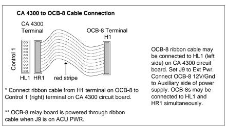
Figure 34 - Terminate Auxiliary Output CA 8300
