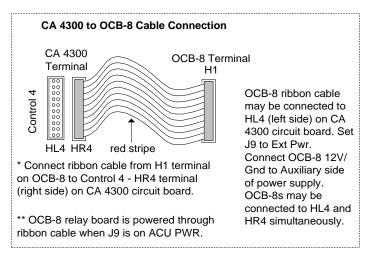
Figure 110 - Handicap Relay CA 8300/OCB-8 Connections
