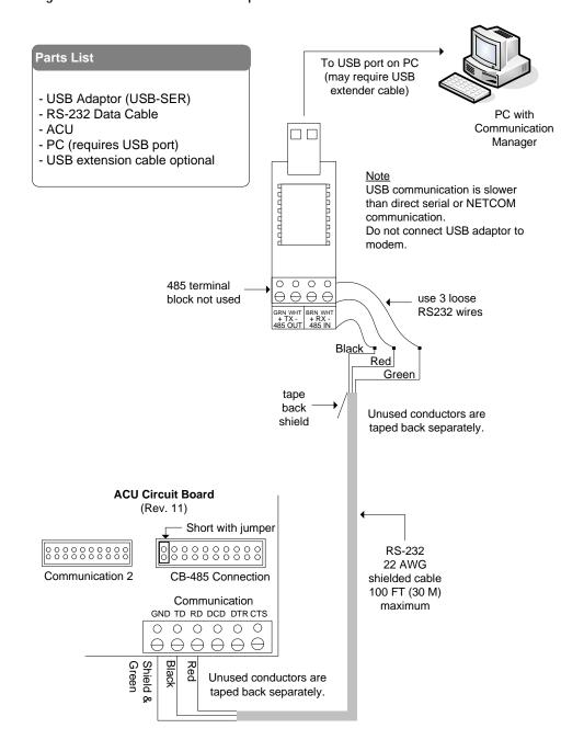
Figure 48 - Single ACU Communication - USB Adaptor/CB-485 (RS232)
