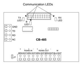
Figure 77 - Communication LEDs on CPB-10
