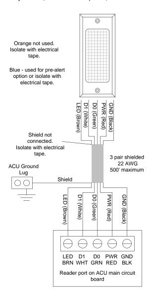
Figure 85 - Keyscan K-KPR Keypad / Proximity Reader (125 KHz HID compatible)
