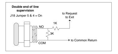
Figure 25 - Terminate Input Wiring - RTE PIR Motion Sensor CA 230 / CA 4300 / CA 8300
