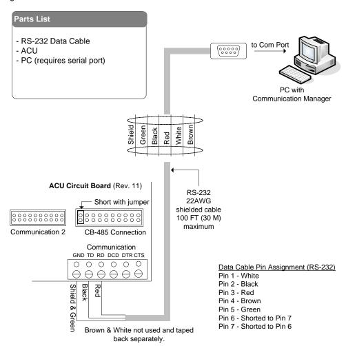
Figure 45 - Single ACU Communication - Serial CB-485
