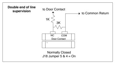
Figure 24 - Terminate Input Wiring - RTE Push Button CA 230 / CA 4300 / CA 8300
