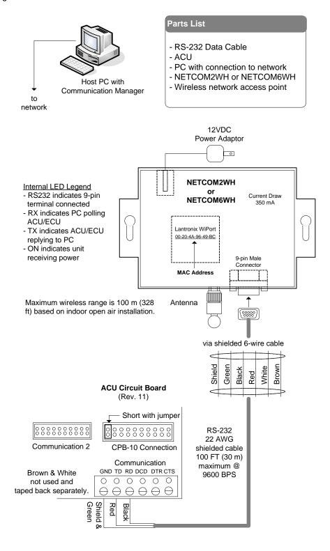
Figure 58 - Single ACU Communication - CB-485M/MC33H
