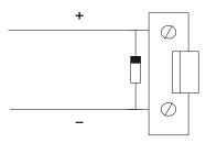
Figure 15 - Typical Door Maglock Connection
