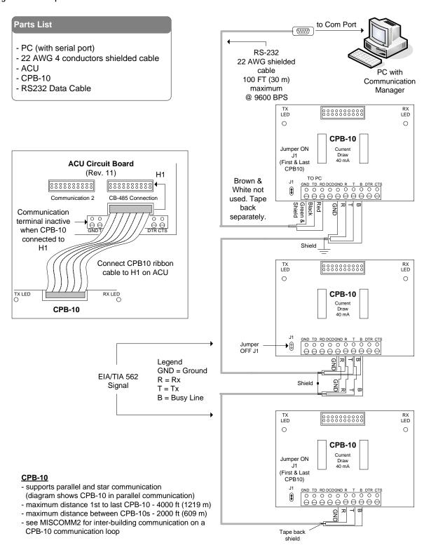
Figure 63 - Multiple ACU Communication - USB Adaptor/CB-485 (RS-232)
