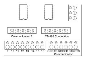
Figure 81 - CB-485 Communication Test Points
