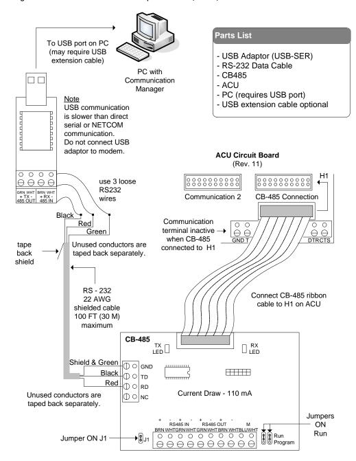
Figure 49 - Single ACU Communication - USB Adaptor/CB-485 (RS485)
