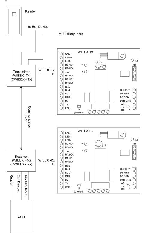
Figure 105 - WIEEX RS485 Transmitter/Receiver Connections
