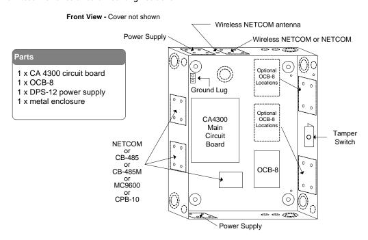
Figure 8 - CA 8000 with Circuit Board Mounting Positions
