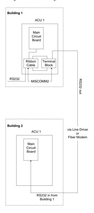
Figure 115 - MISCOMM2 Connections - to a single ACU
