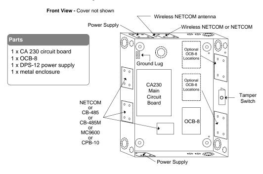
Figure 7 - CA 4000 with Circuit Board Mounting Positions
