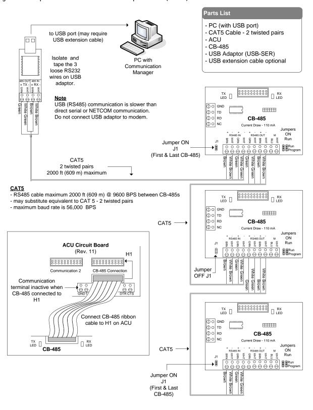
Figure 65 - Multiple ACU Communication - USB Adaptor/CPB-10
