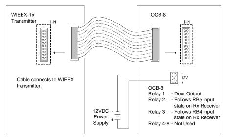
Note: Relays 4 to 8, set jumper J4-J8 to reversed state
