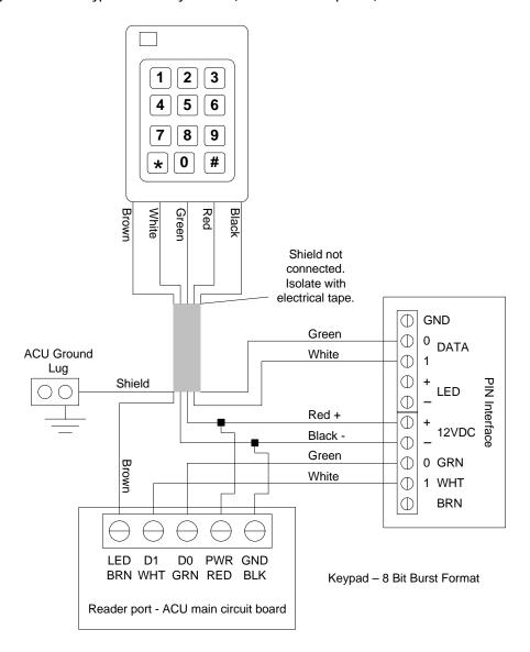
Figure 86 - HID-5395 Wiring
