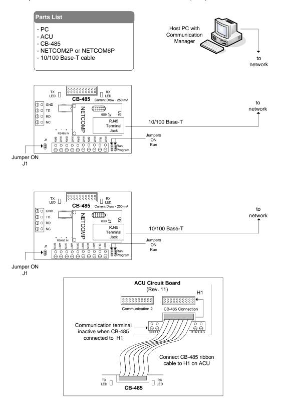
Figure 69 - Multiple ACU Communication - NETCOM2 or NETCOM6 (1 per ACU)
