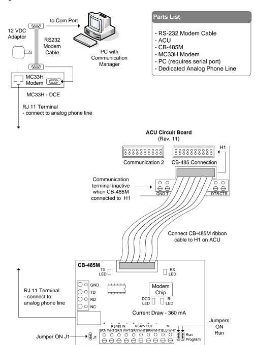
Figure 59 - Single ACU Communication - MC9600/MC33H
