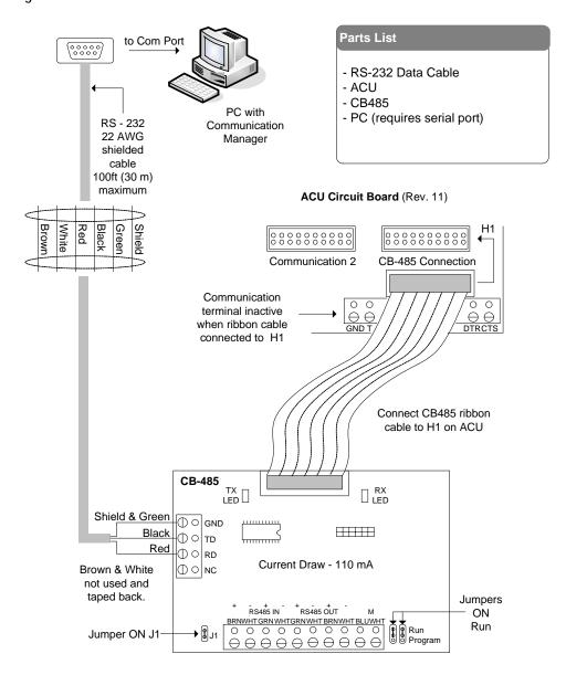
Figure 46 - Single ACU Communication - Serial CPB-10
