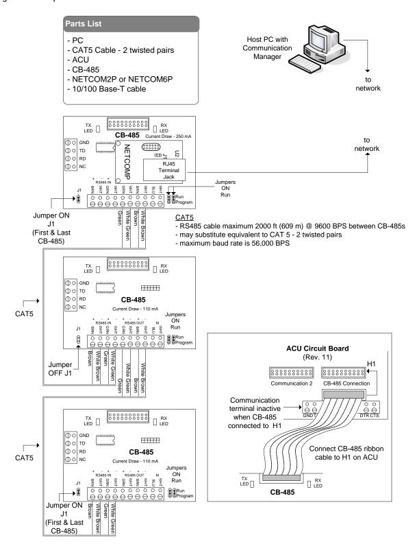
Figure 67 - Multiple ACU Communication - NETCOM2 or NETCOM6/CPB-10
