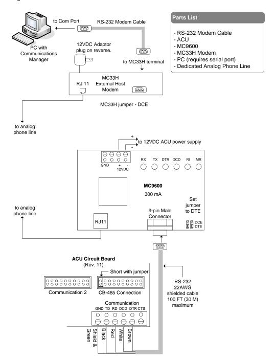
Figure 60 - Single ACU Communication - MC9600/MC33H/CPB-10
