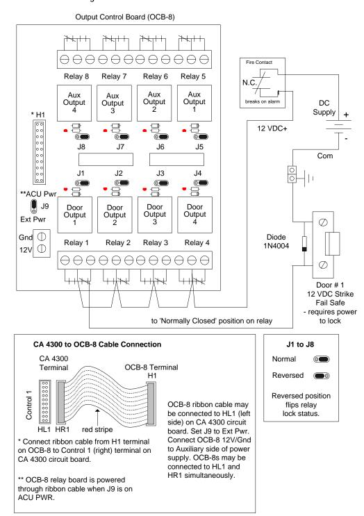
Figure 22 - Terminate Lock Wiring CA 8300
