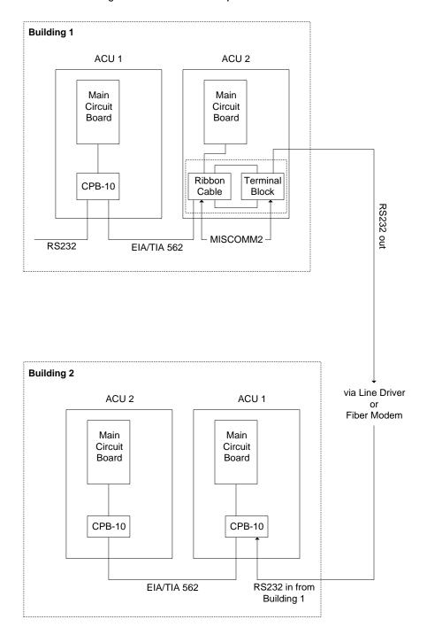
Figure 117 - MISCOMM2 Connections to Multiple ACUs
