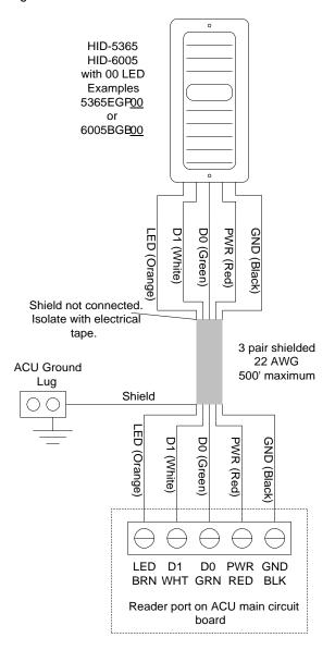
Figure 88 - HID 5355 Wiring
