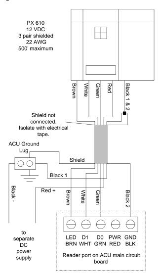
Figure 97 - Indala PX 620 Wiring
