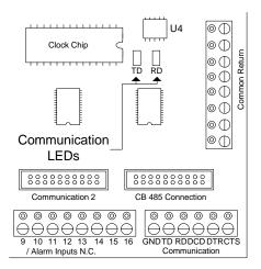
Figure 76 - Communication LEDs on CB-485
