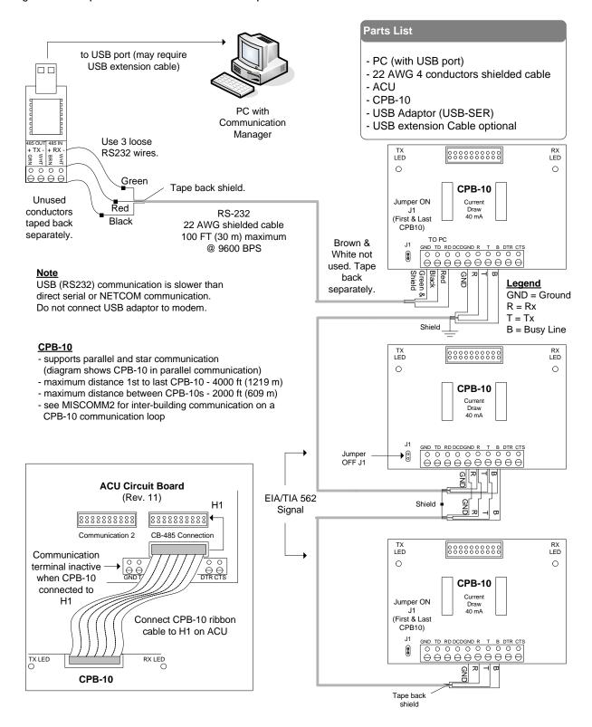
Figure 66 - Multiple ACU Communication - NETCOM2P or NETCOM6P/CB-485
