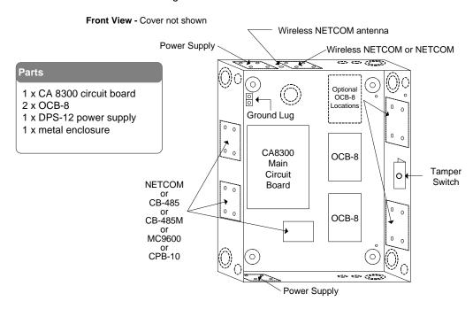
Figure 9 - EC 1000 with Circuit Board Mounting Positions
