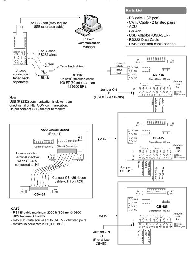
Figure 64 - Multiple ACU Communication - USB Adaptor/CB-485 (RS-485)
