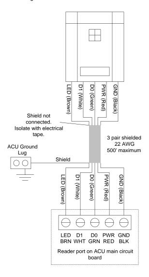
Figure 96 - Indala PX610 Wiring
