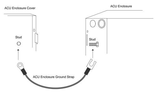
Use enclosed star washers and nuts to secure both ends of cable to studs as shown below.
