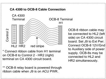
Figure 113 - Pre-alert Relay CA 8300/OCB-8 Connections
