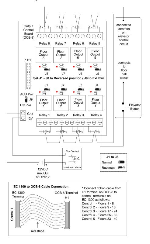
Figure 28 - Terminate Floor Wiring EC 2300
