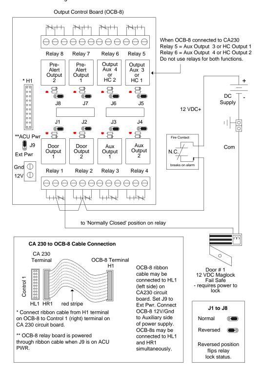
Figure 21 - Terminate Lock Wiring CA 4300
