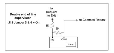
Figure 26 - Terminate Input Wiring - Auxiliary/Supervised Inputs CA 230 / CA 4300 / CA 8300
